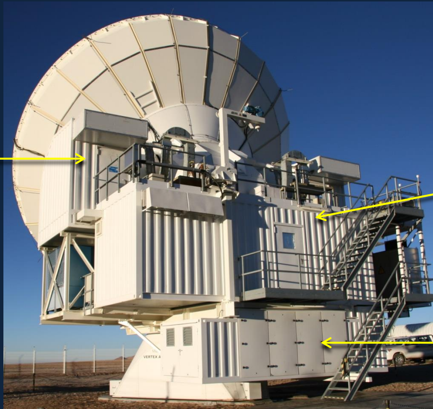
instrument cabin compressor level
